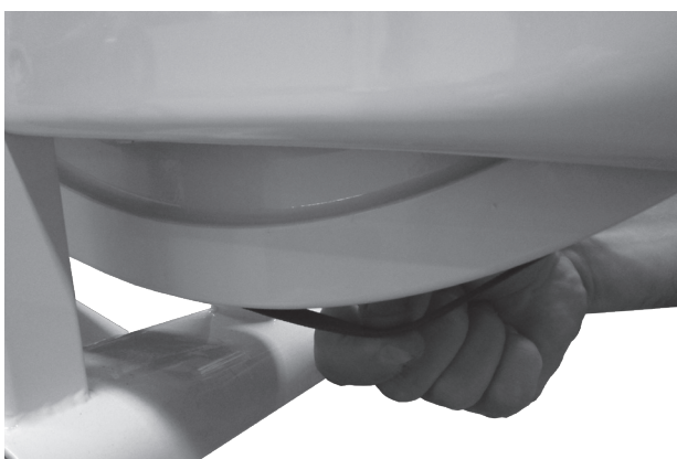
Fig: Control loose brake belt
